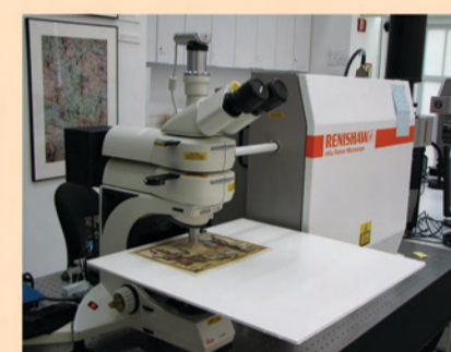
The print Callao de Lima 17th c. under the microscope objective of the Renishaw InVia Raman spectrometer
