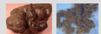
Two mineralogical species of hematite (left) and goethite (right) very commonly used by Prehistoric man in Cave paintings.
