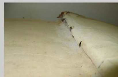
The gray powder collected throughout the gutter of the book for analysis and characterization
